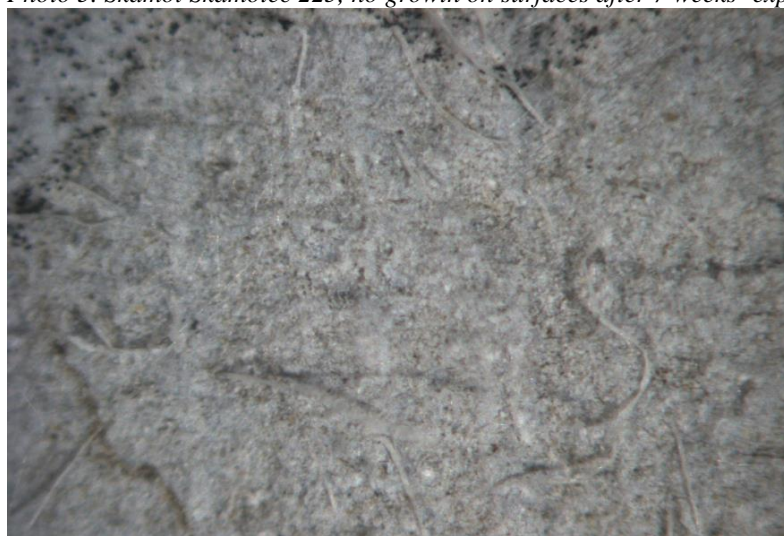
Photo 6. Skamol Skamotec 225, no growth observed in microscope.
