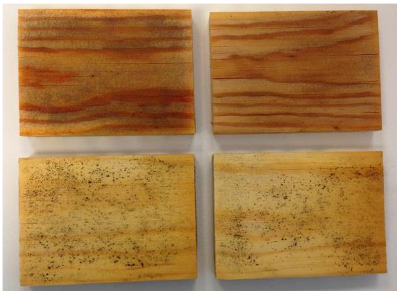
Photo 9. Pine sapwood, growth on surfaces after 7 weeks' exposure
