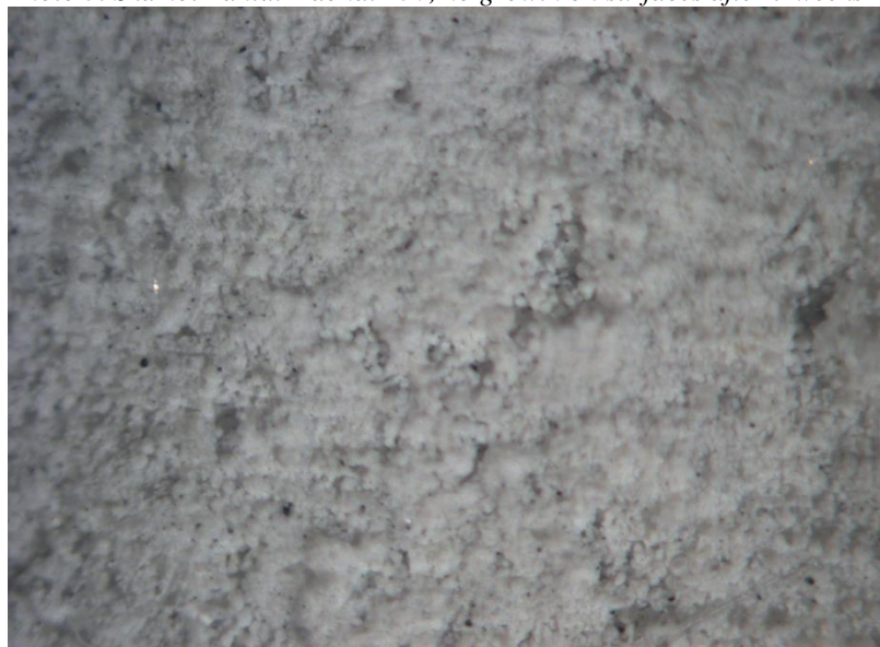
Photo 4. Skamol Yantai Haohai 130, no growth observed in microscope.
