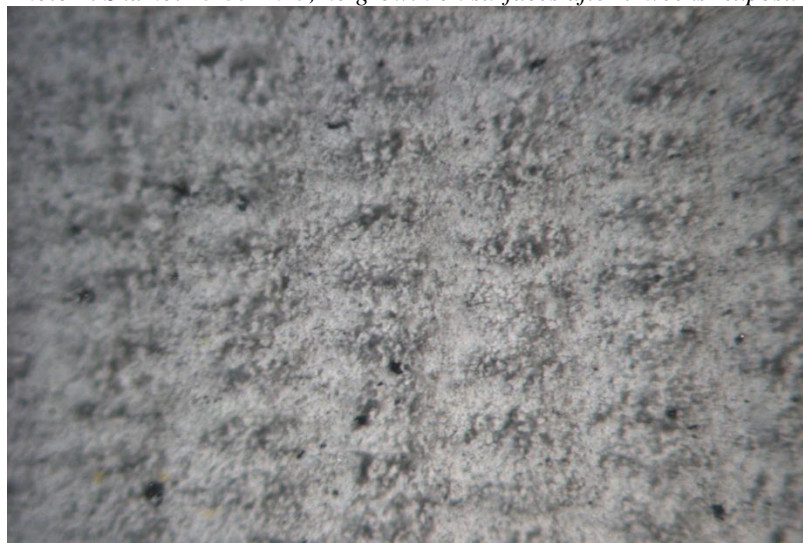
Photo 2. Skamol 15-37-10-3, no growth observed in microscope.
